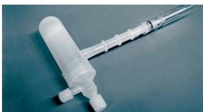
**Option gas line for 7700x.** Suitable for applications that require a mixed carrier gas, such as O<sub>2</sub> for organic solvents or LC mobile phases, and helium carrier gas for laser ablation (standard on the 7700s).
