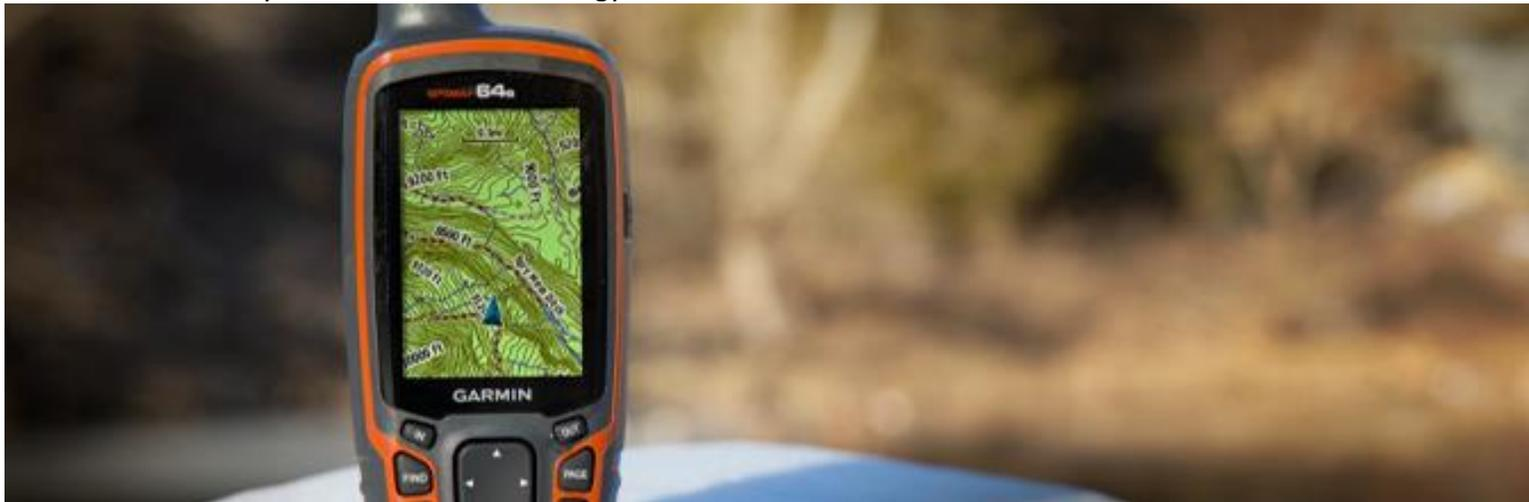
GPSMAP 64s features a 2.6" sunlight-readable color screen and a high-sensitivity GPS and GLONASS receiver with a quad helix antenna for superior reception. GPSMAP 64s includes a 3-axis electronic compass with barometric altimeter, wireless connectivity and a 1-year [BirdsEye Satellite Imagery](#) subscription.
